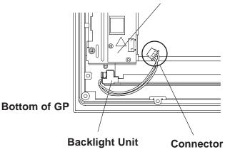
6) As shown here, push the backlight unit's attachment clip to the right to release the backlight unit.
