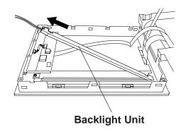
8) Insert the new lower backlight unit into the backlight holder as shown here. After the backlight is completely inserted and the attachment clip clicks into place, lower the unit into the GP.
