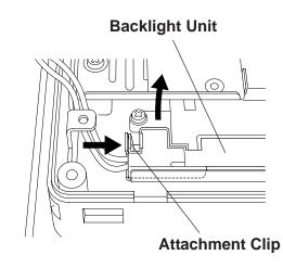
After the backlight unit is released, pull the unit slowly to the left to remove it from the GP unit.
