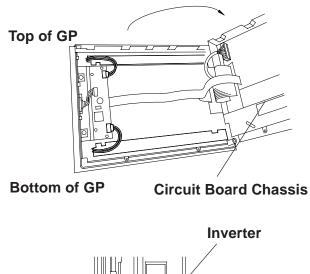
5) Detach the lower backlight unit's power connector from the inverter board.
